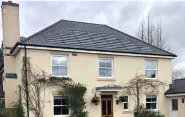
Figure 171: Use of shingle-like solar panels on a slate roof, with the design and colour of the solar panels matching those of the adjacent slate tiles.
